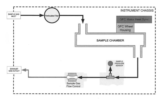
Figure 13-7: Internal Pneumatic Flow – Basic Configuration
